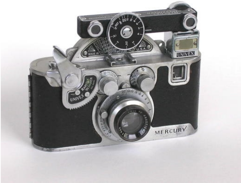
The original Univex Mercury of 1938, decked out with accessory rapid wind lever, extinction light meter, rangefinder and fast f/2.0 Hexar lens.
