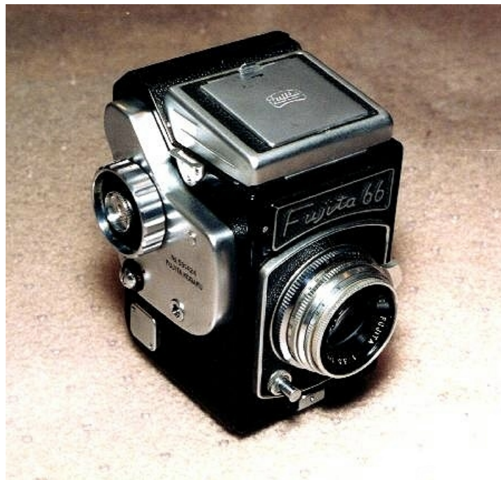
This Fujita 66 of 1958 is identical to my Kalimar Reflex SQ of 1960, except that it lacks the instant-return mirror.
