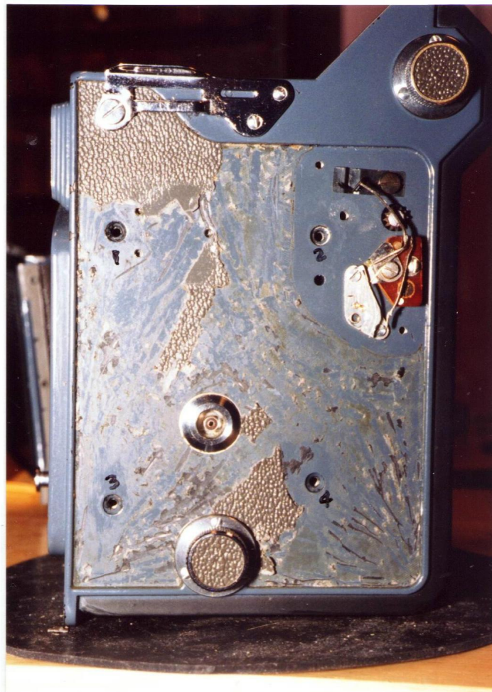
LH Side, 4 screws removed. Synch gear is off and wires pushed inside.
