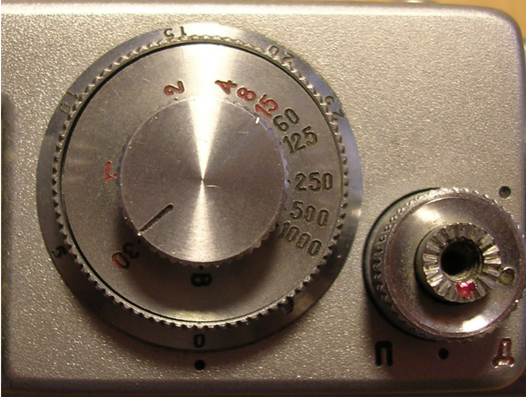
The Zorki 4 shutter speed dial (all speeds)
